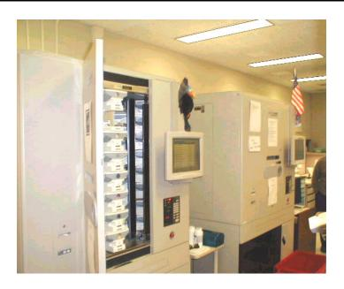
The robots are metal cabinets, approximately six feet high, five feet wide and four feet deep. There are 520 cells which each hold between 100 and several thousand pills. Based on a computer program and a database of prescriptions, the robot will rotate the cells until the appropriate individual pills are above the dispenser and dropped into plastic bags. The bags are sealed, and the inmates' names and time of dispensation are entered.
